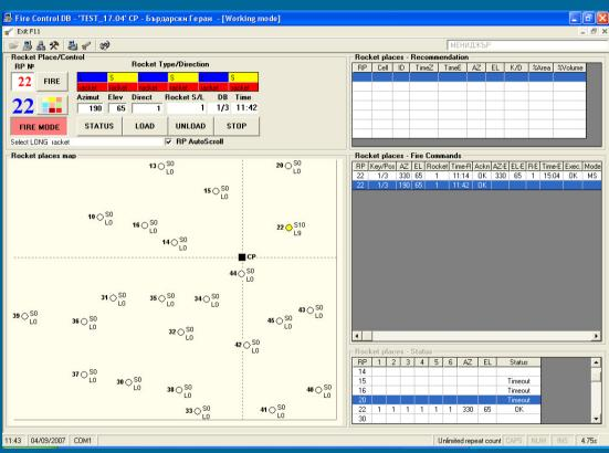
FIRE W – multifunctional software, which carries out many operations: from setting access rights to the system, through a procedure for loading rockets or rocket imitators for training to real work mode and reporting the status of launching sites.
