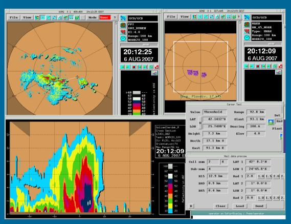
MRL5-IRIS – performs display of cloud systems and selection of hail-dangerous cells, which enables the
