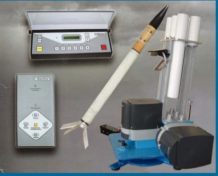
Remote control board – used for checking the launcher, for testing of rockets and firing them. It establishes communication by radio channel with the Control board at the Command post. It records all the gunner's actions during training and firing.
