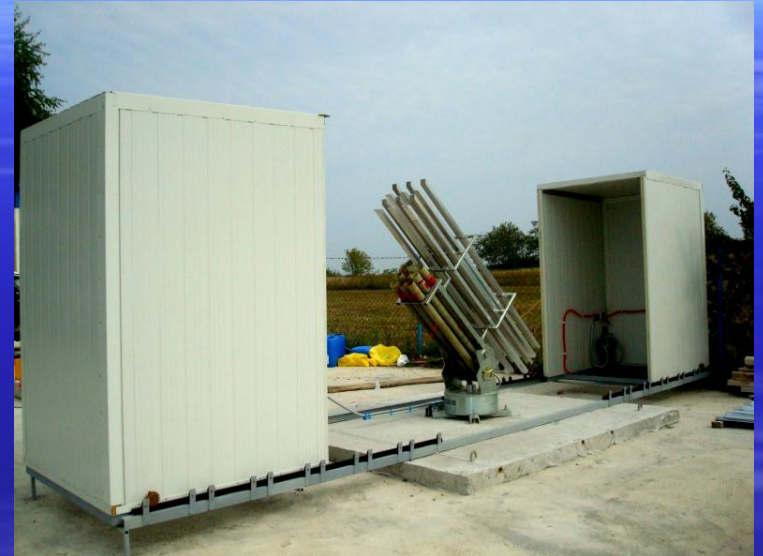
Remote controlled launching station
