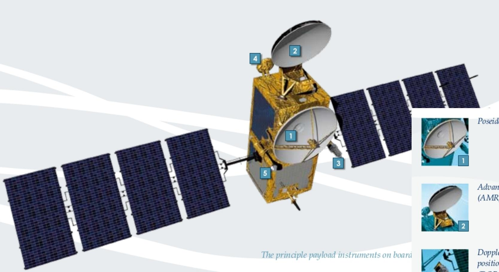
Poseidon-3 dual frequency altimeter
